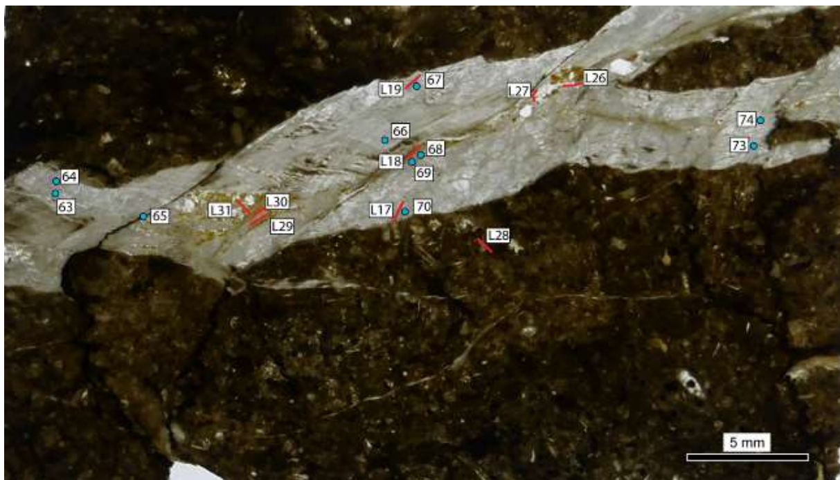
Figure S2 Sample PA3.21. Structural set: CT slickenfibers. Calcite generation: Cal-1 “type”.
