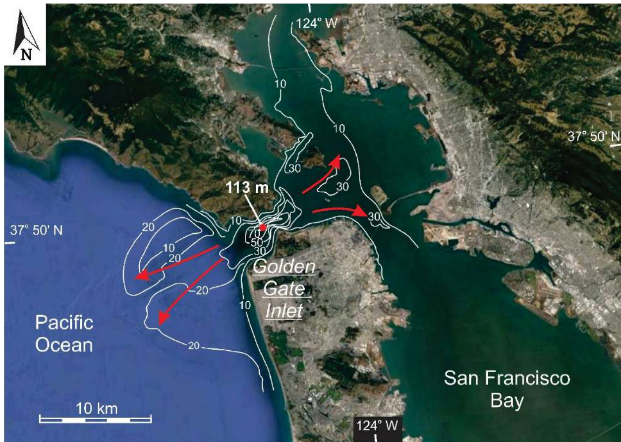
Fig. A5. The Golden Gate Inlet, San Francisco: The bathymetry shown is modified from Rubin & McCulloch (1980, fig. 1C, based on data from the U.S. Coast and Geodetic Survey) for the main inlet throat and within San Francisco Bay, and from Elias & Hansen (2013, fig. 1) for the ebb-tidal delta seaward of the Golden Gate Inlet. Copyright Elsevier; used with permission. Depths in metres. Satellite image from Google Earth ©. (Data: SIO, NOAA, U.A. Navy, NGA, GEBCO, CSUMB SFLM, CA OPC). The deepest depth in the centre of the inlet scour is 113 m below sea level. There is a well-defined ebb-tidal delta at the seaward end of the strait (Hanes & Bernard 2007; Bernard et al. 2013a; Elias & Hansen 2013). The corresponding flood-tidal delta is not clearly evident because San Francisco Bay is relatively filled with sediment. Sediment transport is dominated by tidal currents, that are superimposed on a net seaward transport that is presumably driven by the freshwater discharge of the rivers feeding San Francisco Bay (Erikson et al. 2013).
