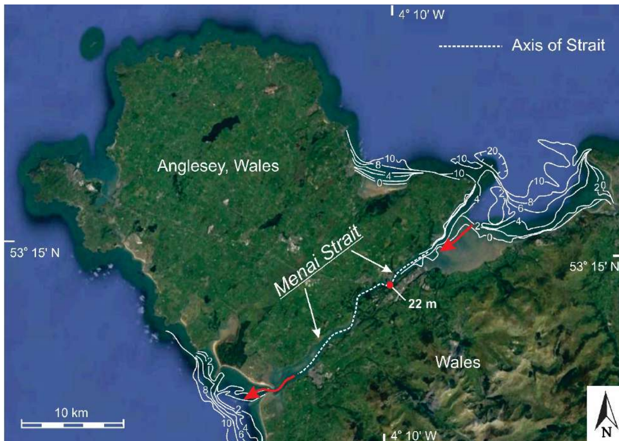
Fig. A14. Menai Strait: Bathymetry modified after Davies & Robins (2017, fig. 1a; copyright Elsevier; used with permission). Depths in metres. Satellite image from Google Earth ©. (Data: SIO, NOAA, U.S. Navy, NGA, GEBCO. Image: CNES/Airbus). No systematic bathymetric data were obtained for the full length of the Strait itself. The Strait is interpreted to occupy coalesced, lowstand fluvial channels. Estuaries occurred at the ends of the channel earlier in the transgression (Roberts et al. 2011). A wave-dominated, barrier-inlet system occurs at the southern end, because of exposure to strong wave action, whereas a tide-dominated system occurs at the northern end, because of sheltering from the strongest waves by Anglesey. Strong tidal currents occur along the entire length of the Strait, but phase differences between the two ends of the channel generate a southward-directed residual current (Harvey 1968; Campbell et al. 1998; Davies & Robins 2017).
