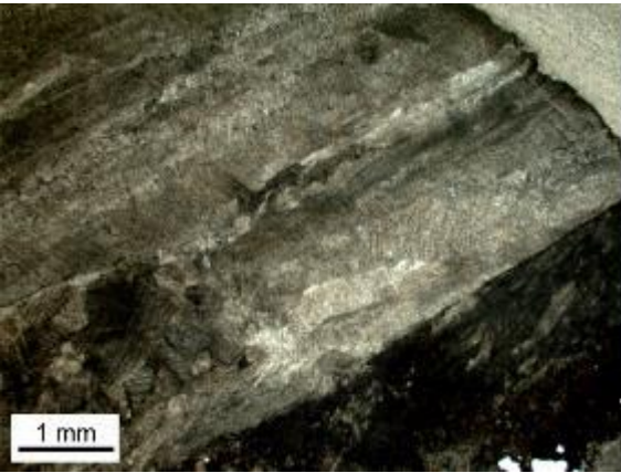
Sample P2: Optical microscope image showing elongated sparite texture parallel to fracture walls.
