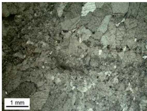
Sample P9: Optical and cathodoluminescence microscope images showing bladed and blocky textures of the analyzed calcite cements.
